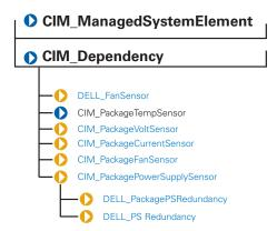
Each class derived from CIM Dependency has an element called an antecedent that represents the independent object in this association, and another element called a dependent that represents the object that is dependent on the antecedent. For example, consider two managed system elements: Chassis and PowerSupply3. Chassis is the antecedent element because a managed power supply would always be either contained in, or grouped with, a chassis.
